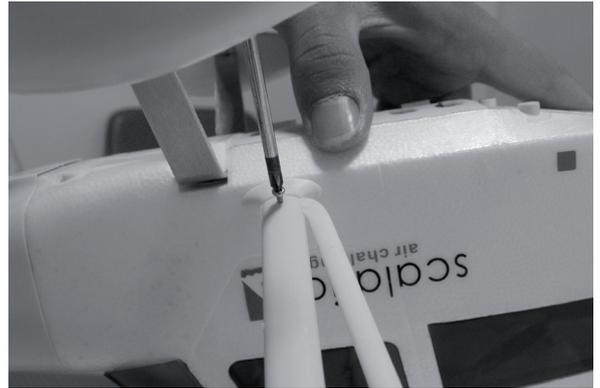
The wing struts are attached to the fuselage and wing with screws.
