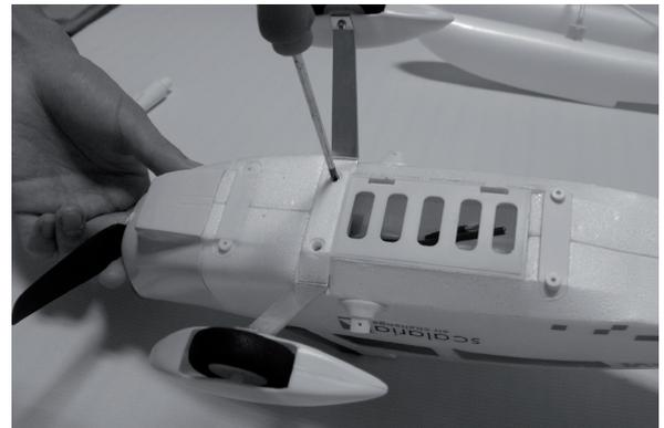
Assemble the main landing gear using the screws included with the scope of delivery.
