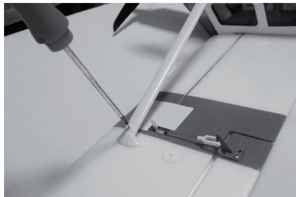
The wing has to be attached to the fuselage using the supplied screw. Plastic wing struts will give additional stability to the main wing structure.
