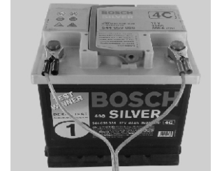
Using terminal clip attaching to car battery
